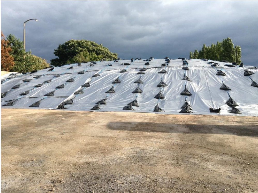
Figure 10: Strategic salt stock under lightweight plastic sheeting (Compass Minerals, England)
