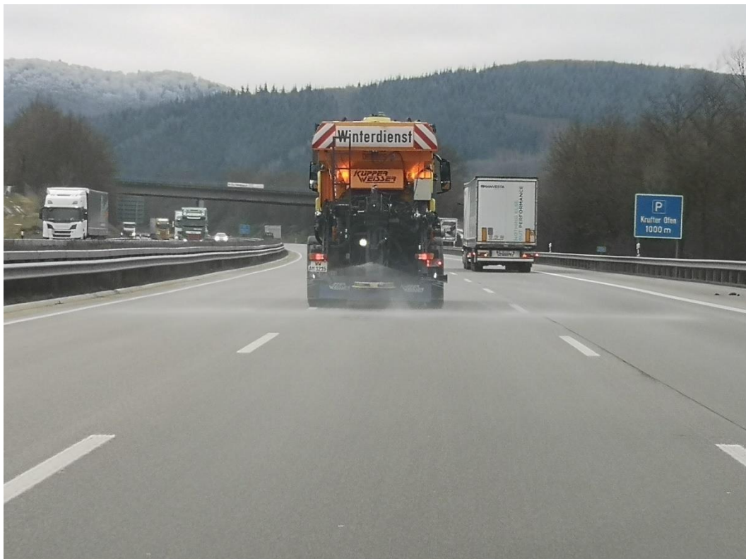
Figure 37: Preventive direct brine application on the German highway A61 (February 9, 2021)
